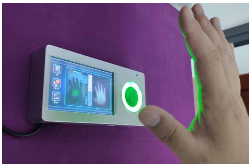
Figure 3. The CUHKSZ touchless palmprint and palm vein acquisition system
